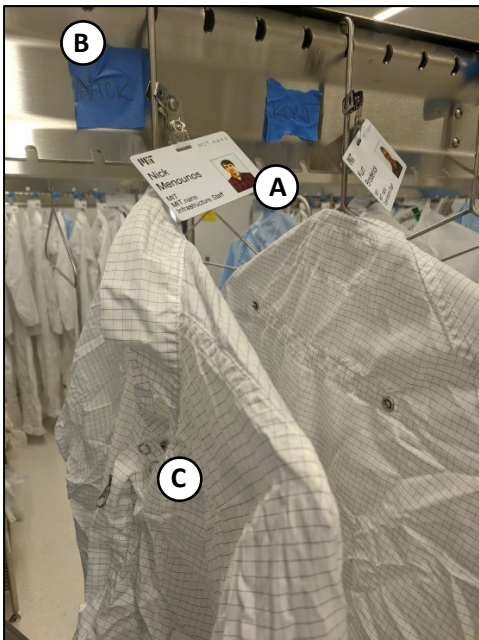
Label hangers with either nametags (A) and/or blue tape with coral username (B). The hood should be clipped inside the suit (C).
